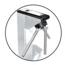
Through an anti-panic mechanism the arm drops leaving the access free. This special feature can be used in emergency cases (activated through a push-button or system in a control room) or in case of power failure (when the turstile does not have the no-break system). The turnstile can also inform the system when the arm drops.
